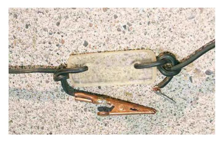
Each length of each segment is measured, cut, and installed sequentially; resulting in the following lengths from the middle of the center insulator to the MIDDLE of each insulator. Allow about 1 extra inch of wire for the securing knot.
