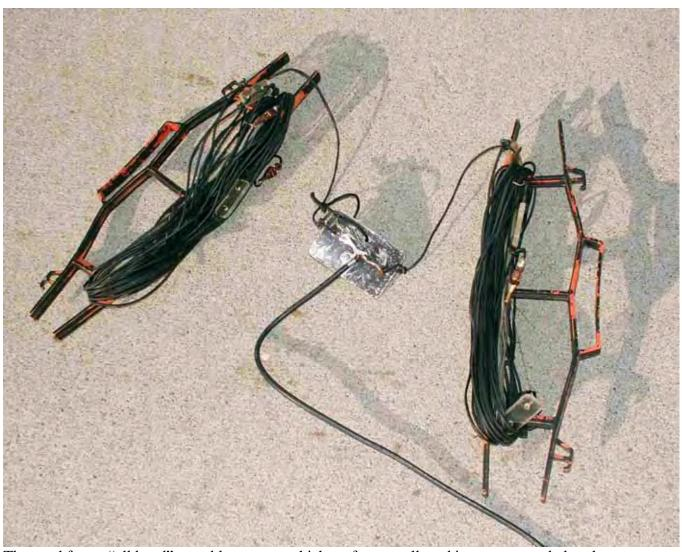
The need for an "all band" portable antenna which performs well, and is easy to use, led to the development of the following wire antenna. It works, without needing a tuner, on the 80, 75, 40, 30, and 20 meter bands.
