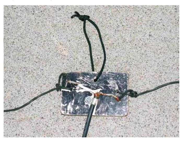
The center insulator is a piece of 1/8 inch thick masonite, approximately 5 x 3 inches. The coax is attached to the center insulator with a small metal clamp, bolted to the insulator. Each side of the antenna is looped through a hole drilled in the insulator, and secured with a knot. All connections are soldered.
