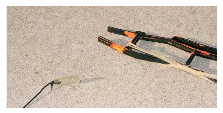
If black zip cord is used, and the insulators and winders are painted flat black, the antenna is mostly "invisible" in a campground. Highly visible flagging should be attached for safety, if necessary.
